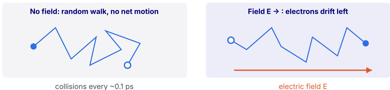
Figure 6.1 A field adds a small, steady sideways bias to the random zig-zag. Collisions with vibrating atoms (phonons) and with dopant ions limit how fast carriers drift, and that limit is what mobility measures.
